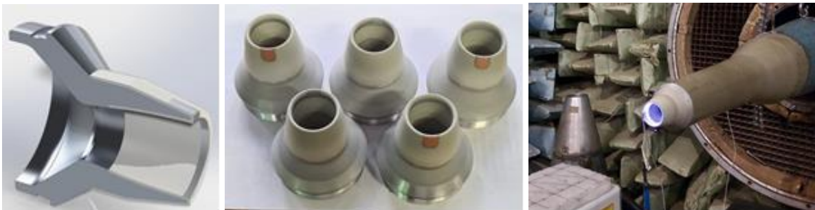
Figure 1. Supersonic nozzles ( M=2 ) with detonation ceramic coating.
